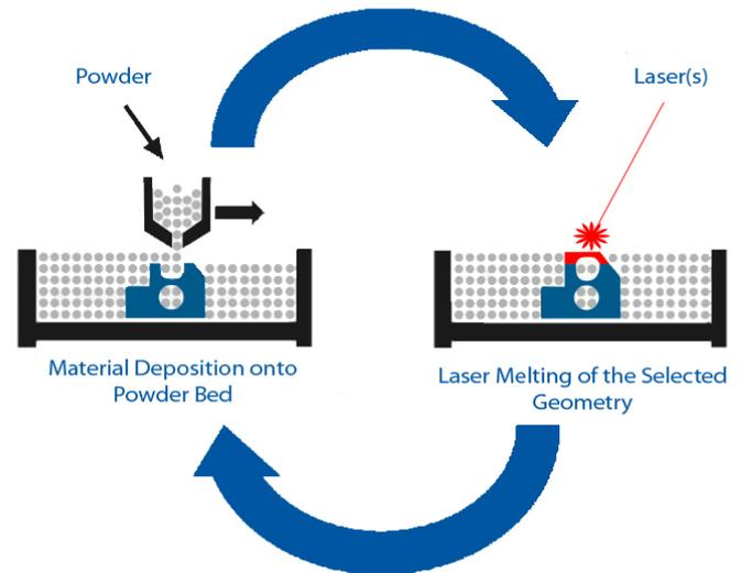
The melting is typically done with a high power laser.
