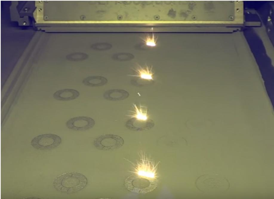
Multiple lasers contribute to increased throughput. Here, four lasers work simultaneously across the build plate to maximize build speeds.
